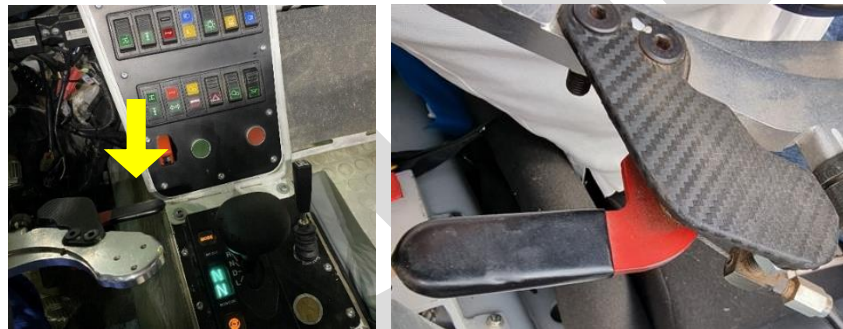
Illustration 1 – Secondary throttle system
