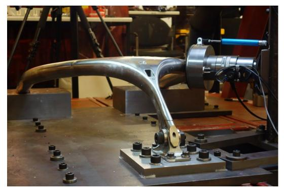
Figure A3.6.3. Example of test equipment for Static Test 3 (Front View)
