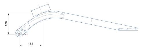
Figure A3.4.1 Load application point for Static Test 1
