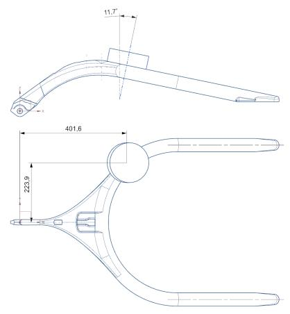
Figure A3.5.1- Load application point for Static Test 2
