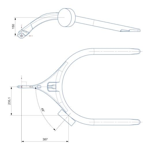
Figure A3.6.1. Load application point for Static Test 3
